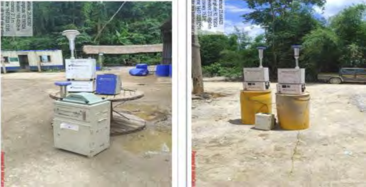
Air Monitoring sample collection from all construction site locations (CP-2).
